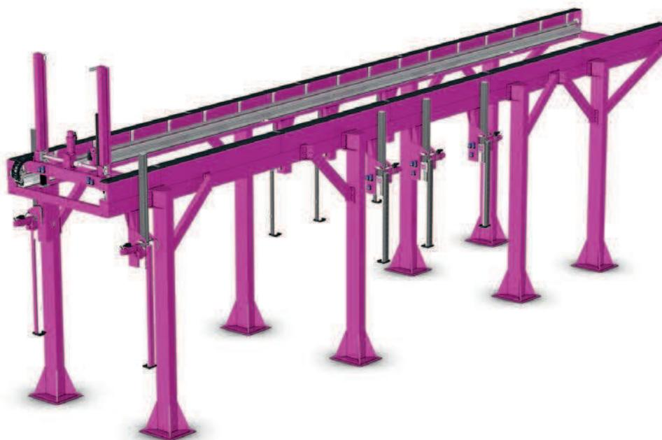
Partial transfer system with lifgo® linear for the horizontal stroke. Scope includes steel construction, assembly, operational testing, and final installation. The grippers take parts from the transfer and dip them into process baths for further processing. Used in the chemical industry.
