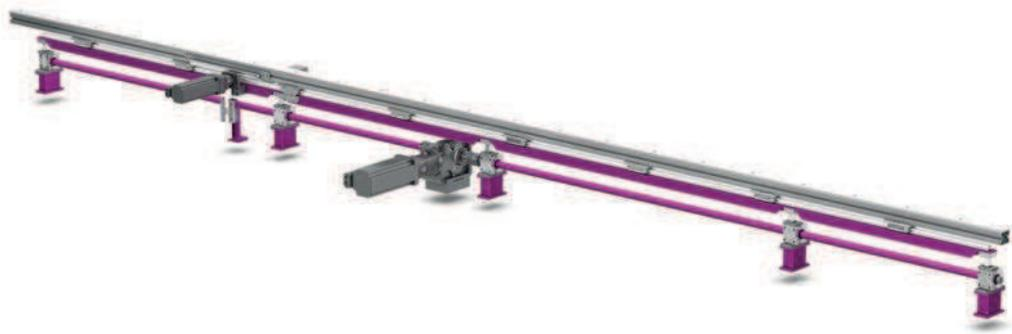
lifgo® gearboxes are oriented vertically in the Z-direction, connected and synchronized by means of the rotary axis. Rotary reinforcements ensure precise angular synchronicity. A lifgo® linear unit with additional lifgo® guide cars is mounted to permit the reverse movement of the profile beam in the X or Y directions. This creates a 2-axis reversing shuttle.
