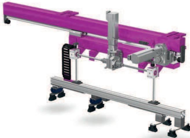
Suspended 1-arm shuttle. The gear rack and lifgo® linear unit for the horizontal drive are suspended below the beam. The assembly and second lifgo® for the Z-stroke are fixed to it. Grippers, suction pads, or other devices can be installed on the suspended standard aluminum profile.
