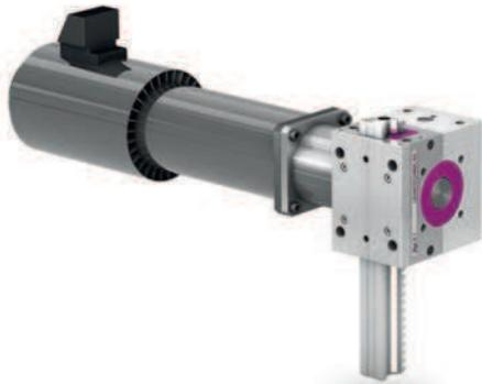
The lifgo® pinion shaft is equipped with pins and a keyway. For precise positioning (horizontal/vertical), the gearmotor is directly connected to the lifgo® pinion using a form-fit coupling. Used as a positioning and adjusting drive, the drive unit can also be used, for example, for pouring and tilting devices.
