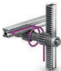
Gearbox combinations basically convert horizontal linear motion into rotation, and then into vertical linear motion. The drive motion can take place in any effective direction (arrow). Reverse operation is also possible.
