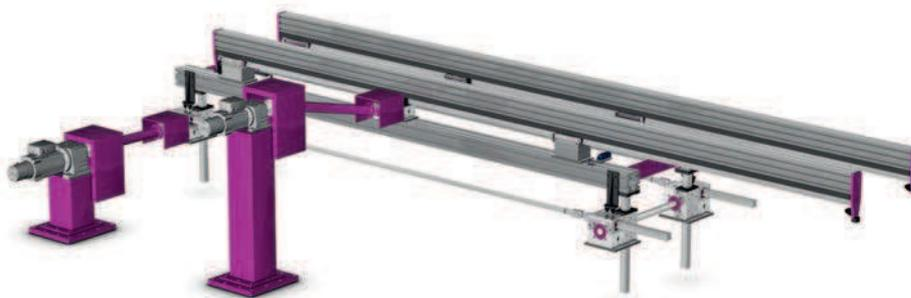
Designed as a 2-axis transfer shuttle with externally mounted drives. The system can also be designed as a 3-axis transfer gripper shuttle.
