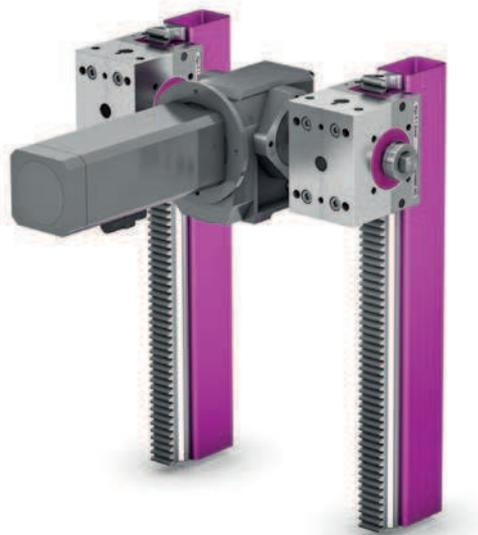
Lift column with particularly rigid design, for lifting heavy parts/fixtures in assembly lines, such as for the final assembly of front axles with engine/transmission in the automotive industry. Large stroke heights, high transverse force capacity and positioning accuracy.
