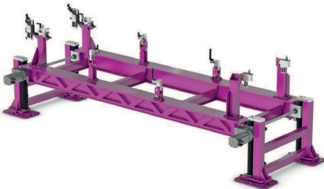
Lift table for high loads with high repeat accuracy. Loose guidance to prevent overdefinition, for example during centering tasks. A lift table consists of two double columns, each of which is equipped with two lean SL® gearboxes and, in the configuration illustrated here which uses size 5.3 gearboxes, is able to lift 1800 kg, for example.
